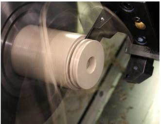
In some cases, we are able to hold  $\pm$ .0005" dimensional tolerances. All products manufactured by Precision Associates are lot controlled and 100% visually inspected for defects. Materials can be virgin or filled for additional strength or to increase wear properties, including self-lubricating options.
